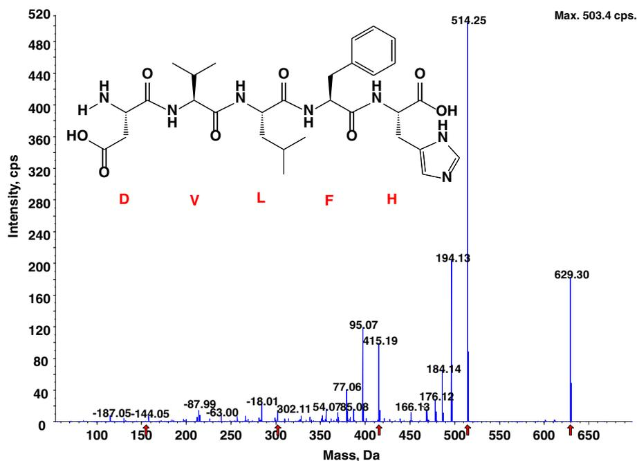
**Fig. 3** Identification of molecular weight and amino acid sequence of the purified peptide from SWH24 by HPLC. MS/MS experiments were performed on a Q-TOF tandem mass spectrometer equipped with a nano-ESI source
