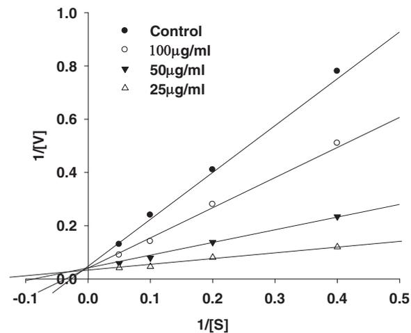
**Fig. 4** Lineweaver-Burk plots for determining inhibition pattern of the purified inhibitor against  $\beta$ -secretase. The intersection of the three lines on the vertical axis signified that the purified  $\beta$ -secretase inhibitor was a competitive inhibitor
