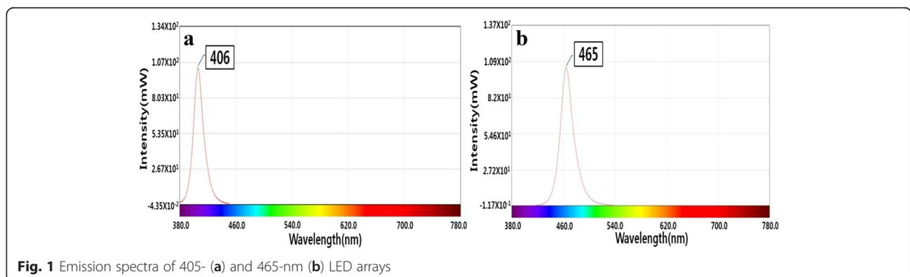
**Fig. 1** Emission spectra of 405- (a) and 465-nm (b) LED arrays
